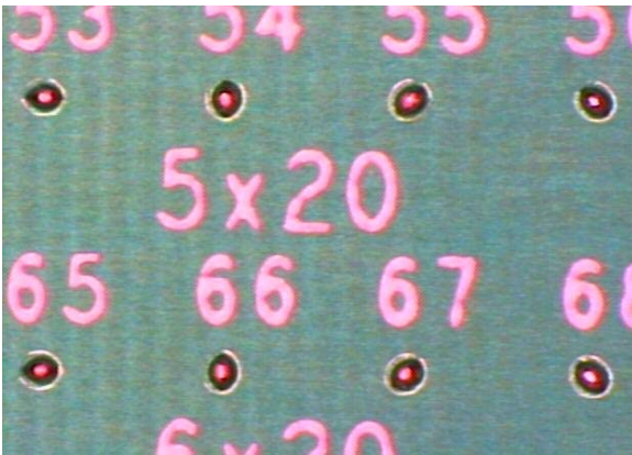
Figure 3. Solder mask-defined solder bead pads
