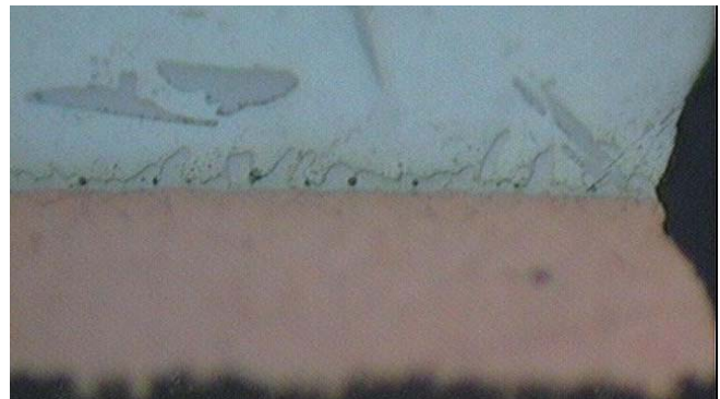
Figure 15: Right side close-up of solder bead and trace—no degradation after aging and 10 probe hits
